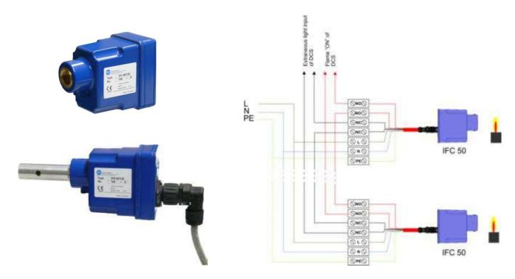
IFC/IFR 50 is a compact UV flame detector\* conceived especially for industrial furnace applications. Its internal relay offers one isolated NC contact and an isolated NO contact with high switching performance. Thus, the IFC/IFR 50 is suitable for multi-flame control with ambient light control. The flame detector IFC/IFR 50 is provided according to the UL Std 372 for firing, which requires a controlled shutdown upon flame signal interruption.
