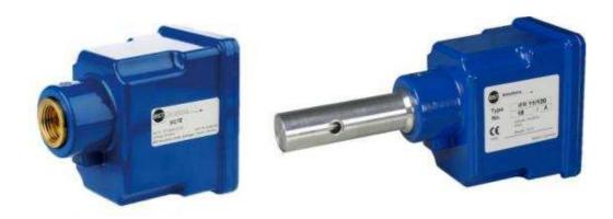
With the diopter holder, which serves also as a mounting of the flame detector to the combustion chamber, the IFC/IFR 10 can be fitted with different glasses and lenses to special requirements. This flame detector is equipped with an optical interface which visibly indicates the flame signal intensity. A simple diagnosis of the flame intensity is directly on the furnace or boiler possible.
