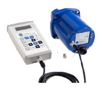
The CFC100 has been designed to monitor gasand oil flames on single and multi burner applications. For the first time with UV tube sensors it is possible to set high-resolution thresholds for flame discrimination. Due to new shutter design with electrical/mechanical combination we increased the shutter lifetime by 20 times. Also the UV tube lifetime was increased by 3 times due to the use of special high-temperature sensors.
